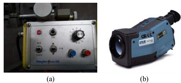
Figure 2: Image of welding speed controller(a) and thermal image camera : Thermal CAM P25(b)
