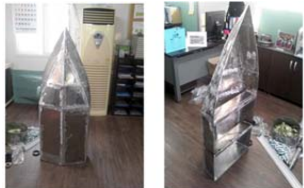
Figure 14: Actual prototype image for Al 5083 co-environmental boat discussed in this study
