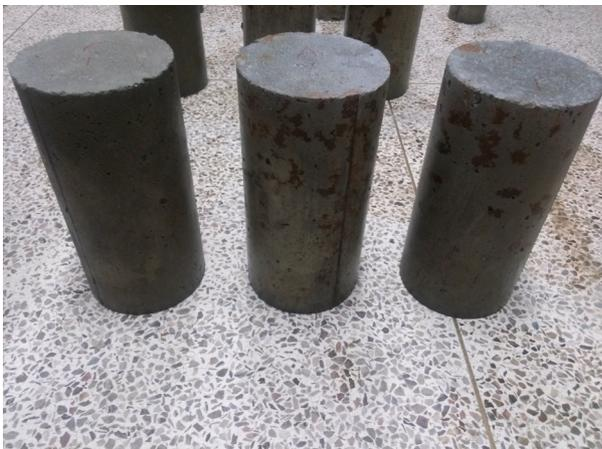
Photo 3. Surface condition of concrete specimen
