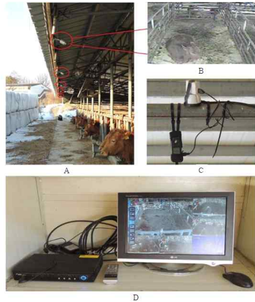
Fig. 2. Closed circuit camera, sound recorder and digital video recorder. A: closed circuit camera, B: an image of barn from closed circuit camera, C: real time recorder, D: digital video recorder monitoring system.
