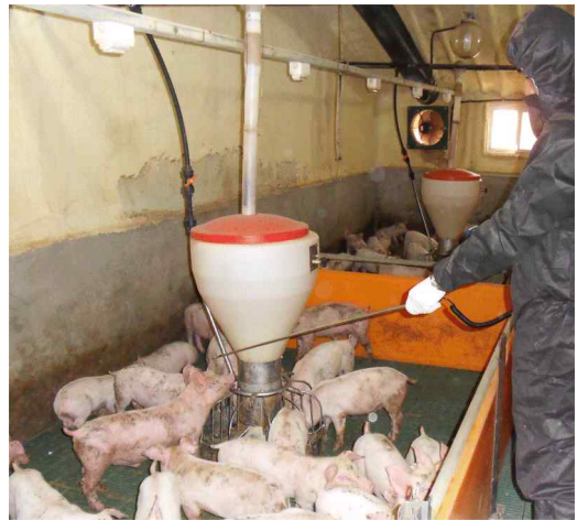
Fig. 4. Measurement of air velocity in pen.
