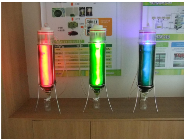
Fig. 6. A tubular photobioreactor with LEDs inside.
