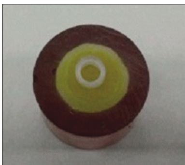
Fig. 2. Composite resin cylinder bonded to a specimen.
