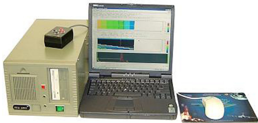
Fig. 5 Intraspect ultrasonic data acquisition and analysis system
