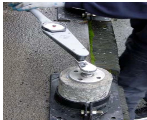
Fig. 5 WDSOT Personal Performing the Torque Bond Test (Al-Qadi, 2008)
