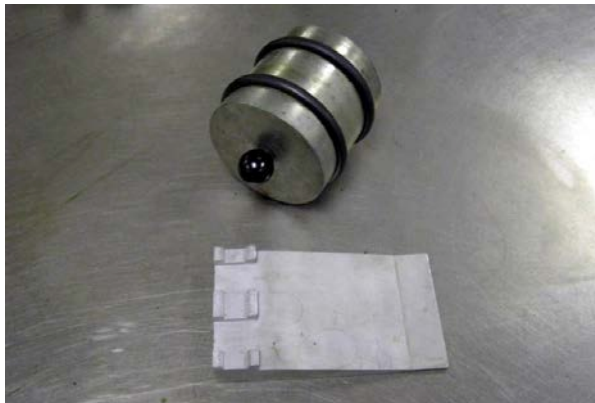
Fig. 3 Tracking/Pickup Device Specified in ASTM D 711 (Clark, 2012)
