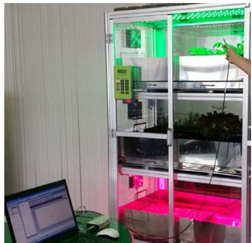
Fig. 1 Measuring wavelength of LED system
