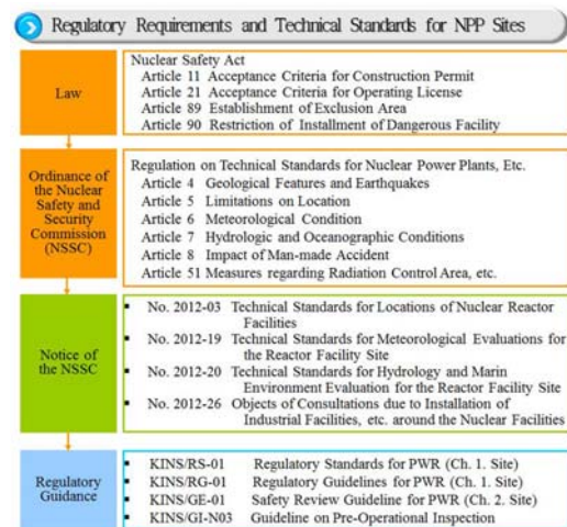
Fig. 2. Schematic flowchart showing the list of regulatory requirements and technical standards applied to nuclear power plant site selection and site evaluation in Korea.
