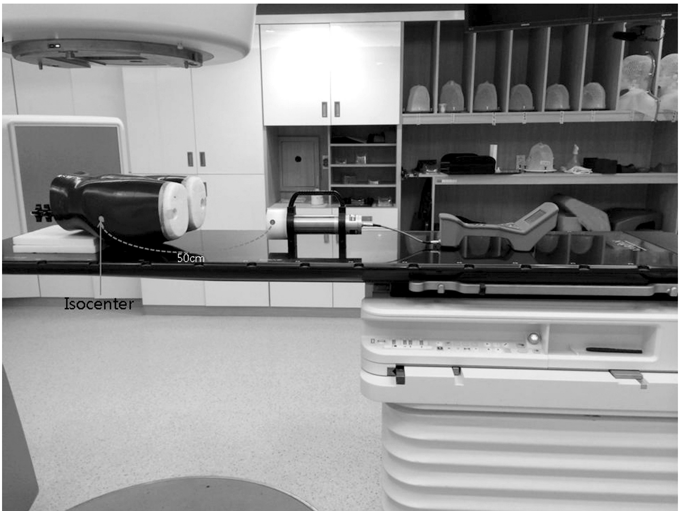
Fig 1. Setup for measuring photoneutron with Surveillance And Measurement 940
