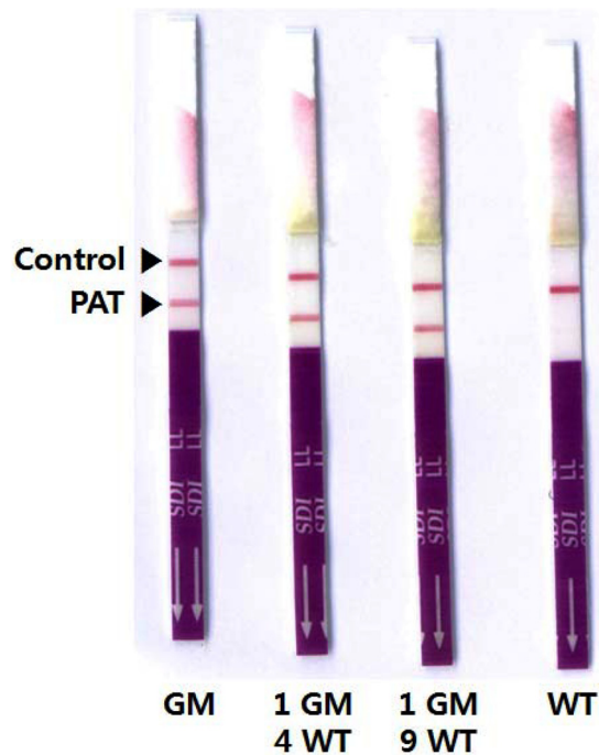
Fig. 1. ImmunoStrip test to detect PAT protein in GM zoysia grass leaf samples. The test was performed with samples of only GM: 1 GM and 4 WT; 1 GM and 9 WT; only WT.
