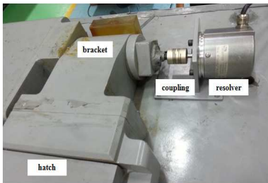
Fig. 15 Backlash measurement of the hatch rotational shaft
