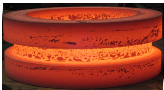
Fig. 8(b) Profile ring rolling test ( \Phi 795 , Filling)
