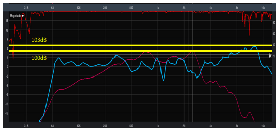
[Fig. 4] Comparisons of the maximum sound pressure level for the magnetic type speaker with variations of magnetic field intensity
