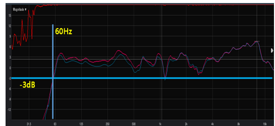
[Fig. 5] Comparisons of the frequency characteristics between the general type speaker and the magnetic type speaker with 2.4 ml
