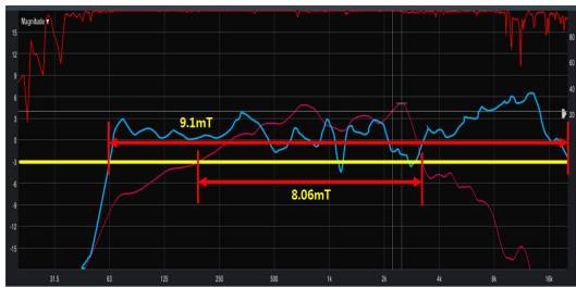
[Fig. 6] Comparisons of the frequency characteristics for the magnetic type speaker with variations of magnetic field intensity
