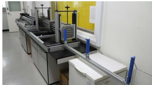
Fig. 1. Fuel rod insertion load test equipment.
