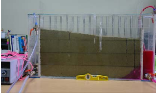
Fig. 9. Experiment result of seawater-freshwater interface.
