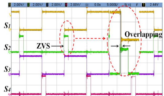
Fig. 14. Gate signal waveform using the proposed method
