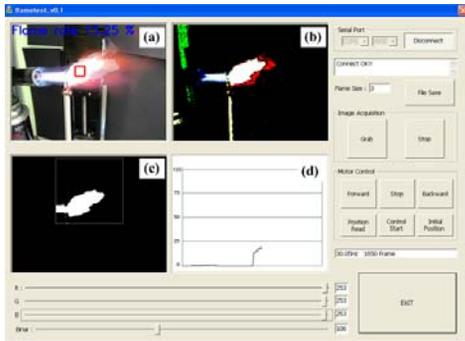
Fig. 8 GUI for the position control from the flame image
