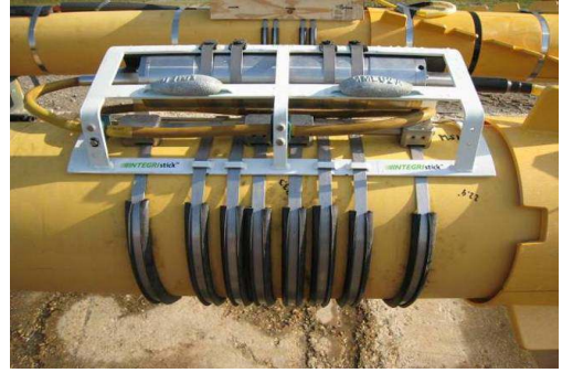
Fig. 7 Motion and Strain Sensors Attached to a Riser
