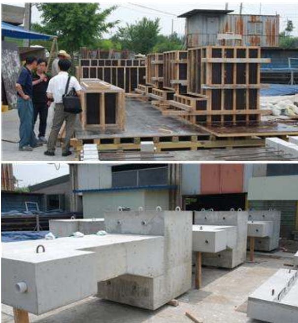
Fig. 8 The View of Form Works and Fabrication of Experimental Specimens
