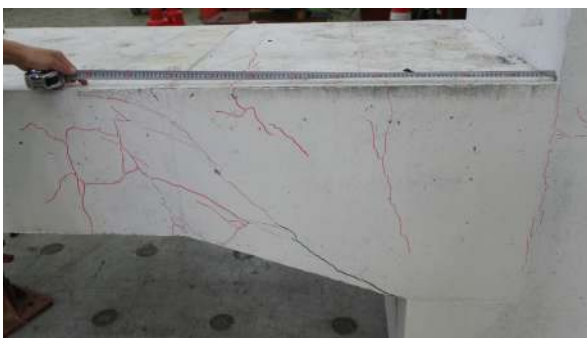
Fig. 21 Crack Pattern of Fix Connection Types
