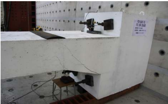
Fig. 20 Structural Failure by Diagonal Shear in Fix Connection Types Specimens
