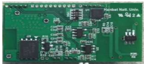
Fig 10. PCB of ZigBee Chip Communication Module for Remote Radiation Measurement (BOTTOM Side)
