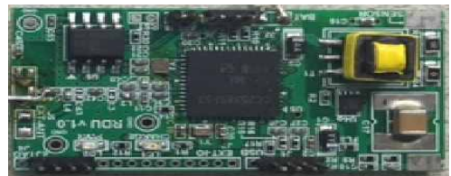
Fig 9. PCB of ZigBee Chip Communication Module for Remote Radiation Measurement(TOP Side)
