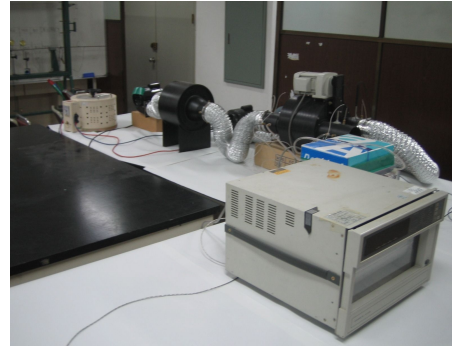
[Fig. 4] Experimental apparatus for heat recovery ventilator with rotating porous disk
