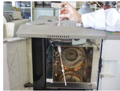
Fig. 3. Spiking of liquid standards onto adsorbent tubes through a GC packed column injector.
