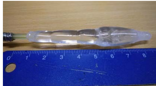
Fig. 1. Photograph of a \text{Li}_6\text{Gd}(\text{BO}_3)_3:\text{Ce}^{3+} scintillator grown by Czochalski method
