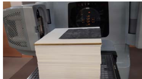
Fig. 2. A photograph of phantom setup used for measuring the shielding ratio of 1 mmPb.
