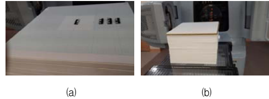
Fig. 1. Photographs of phantom setup used for measuring the off axis ratio. (a) OSLnDs positioned at 2, 4 and 6 cm from the field edge and center axis a radiation field, (b) a solid water slab of 0.5 cm thickness and a bolus of 0.5 cm thickness positioned over the OSLnDs, respectively.
