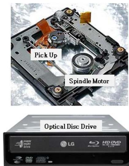
Figure 4. Internal Structure of Optical Disc Drive
