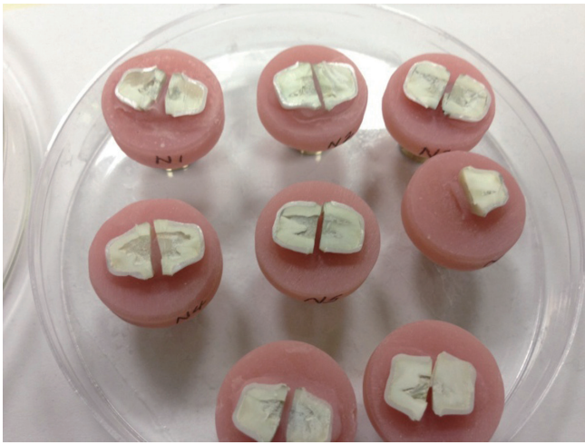
Fig. 1. Sectioned copings mounted in acrylic resin.
