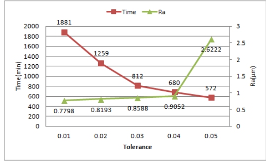
Fig. 10 Flat surface roughness and machining time according to tolerance
