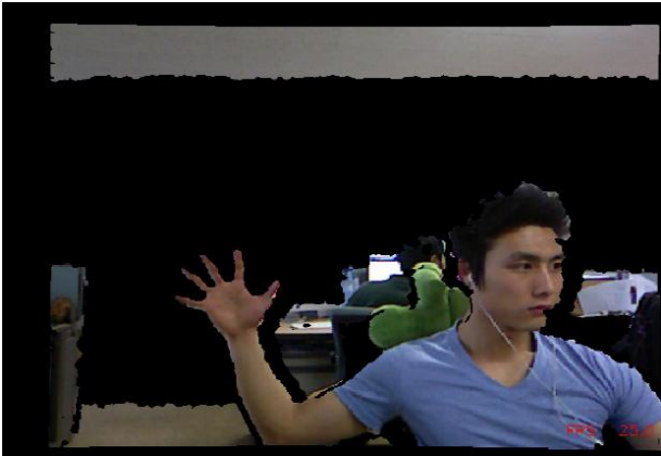
Fig. 3. Mapping the color and depth information with the given function from the Kinect software development kit (SDK).
