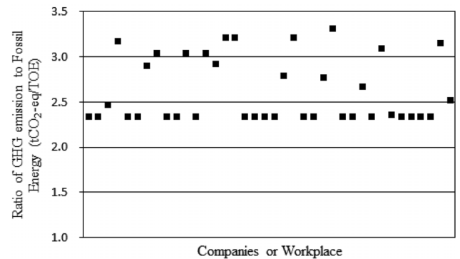
Figure 4. Ratio of GHG emission to fossil energy consumption (The data of 38 companies or workplace are gathered).
