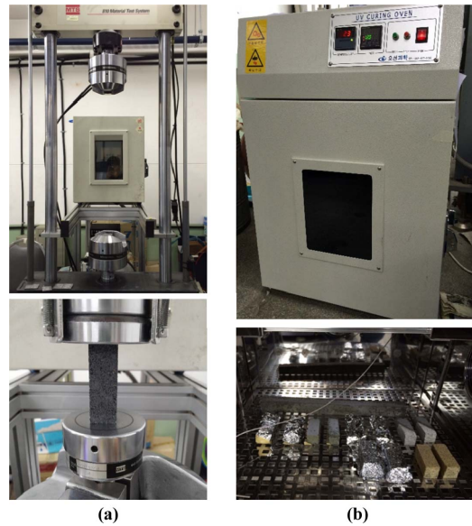
Fig. 1. Experimental test setups; (a) Compressive test, (b) UV exposure test
