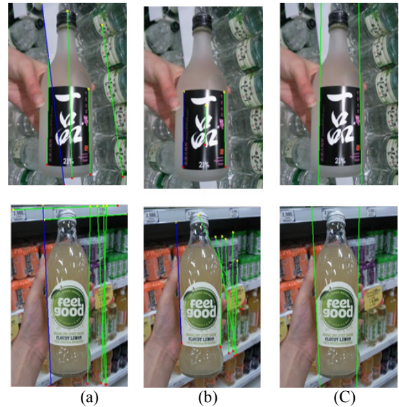
Fig. 9. Comparison of the results of the line detection (a) without and (b) with applying the saliency map, respectively and (c) the final straight line detection results after selecting two similar lines
