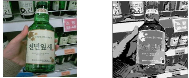
Fig. 3. Gaussian Mixture Model labeling (a) Input image and (b) segmentation result by GMM
