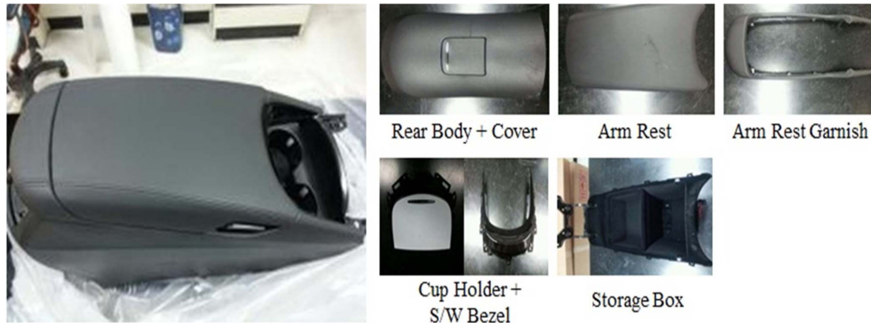
Fig. 4. Console assembly and unit components.
