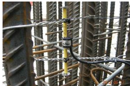
Fig. 2 Vibrating wire strain gauge
