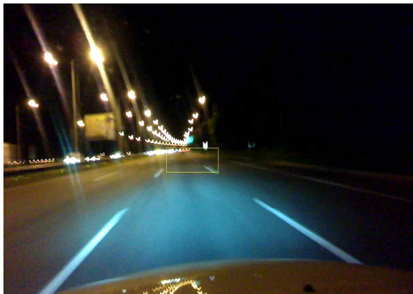
Figure 15. Target Tracking Imagery for Assessment of Road Visibility at Night
