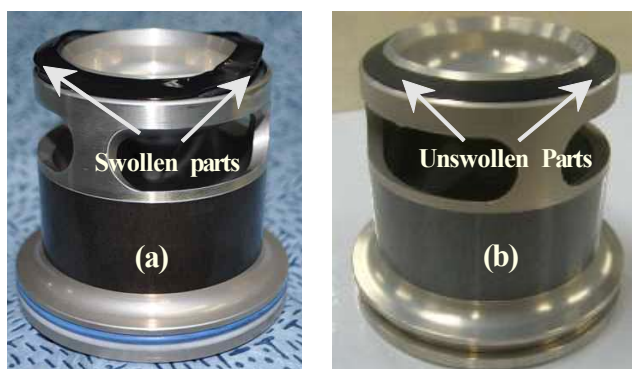
Figure 3. Swelling of (a) the failed and (b) the unfailed packing rubber parts in JP-8 fuel.
