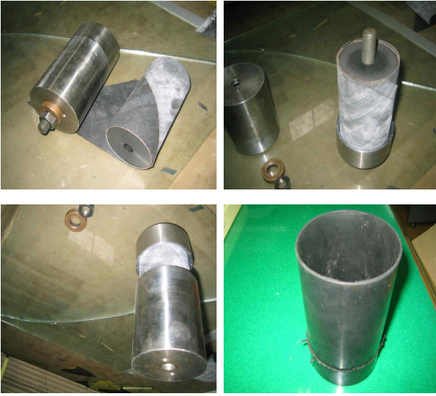
Figure 2. Process of building prototyped rubber sleeve.
