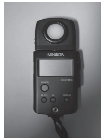
Fig. 2. Color meter used to measure the color temperature.
