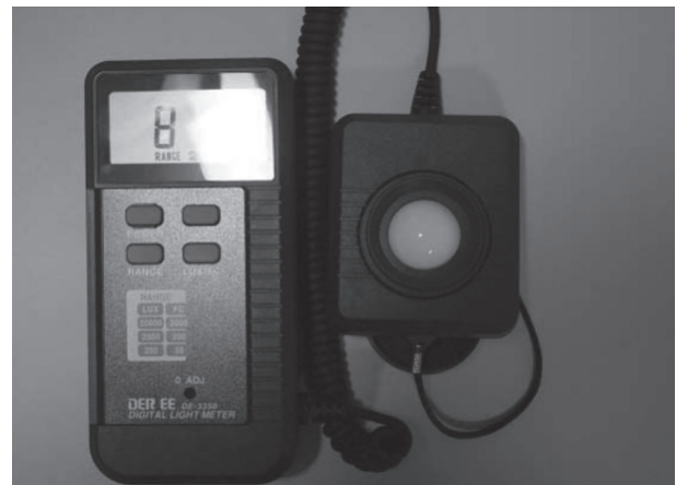
Fig. 1. Lux meter used to measure the luminous intensity.
