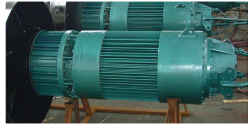
Fig. 5. General view of the large dry submersible induction motor
