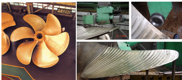
Figure 9. Product of large propeller of ship(diameter : 11m, weight : 114 ton) and 5 axis machining center of Hyundai Heavy Industries
