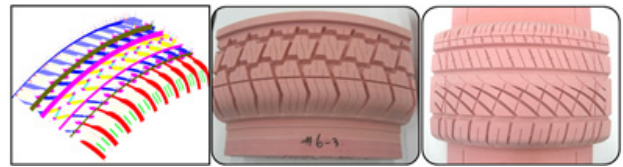
Figure 10. Product of tire master model based on dedicated CAM system
