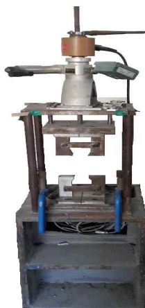
1) Test set-up for tensile strength measurement
