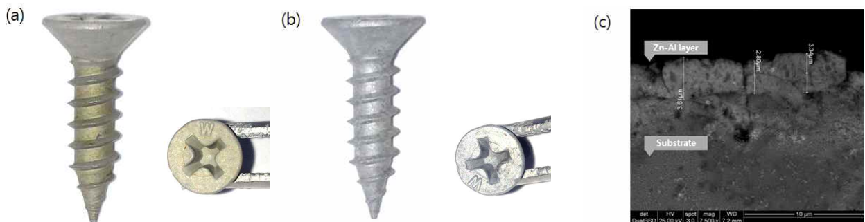
Fig. 7. Screw images before/after Zn-Al thermal diffusion coating. (a) Normal screw body and head before coating process, (b) Zn-Al thermal diffusion coated screw body and head after coating process and (c) cross section of Zn-Al thermal diffusion coated screw. The layer's thickness is about 3 \mu m.
