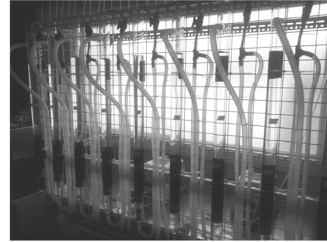
Fig. 4. Pilot plant for GAC test.
