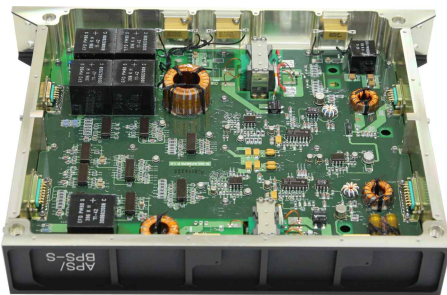
Fig. 9. Anode power supply and bias power supply for the flight model
