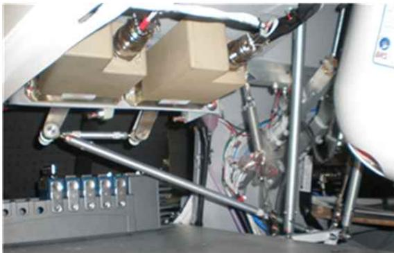
Fig. 7. Aileron control actuator installation
