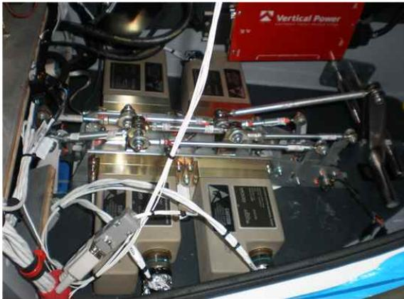
Fig. 6. Elevator and rudder actuator installation
