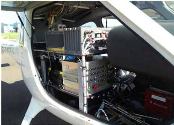
Fig. 10. Onboard system installation rack
