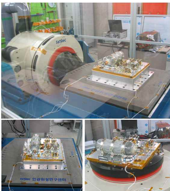
Fig. 4. Test Setup for random vibration test
