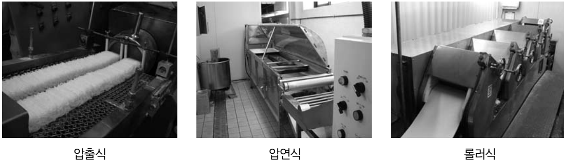
Fig. 3. Rice noodle manufacturing method
