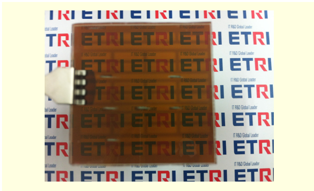
Fig. 4. Photo of penetration-type solar Cell 4 with buffer layers at n/i interface.
