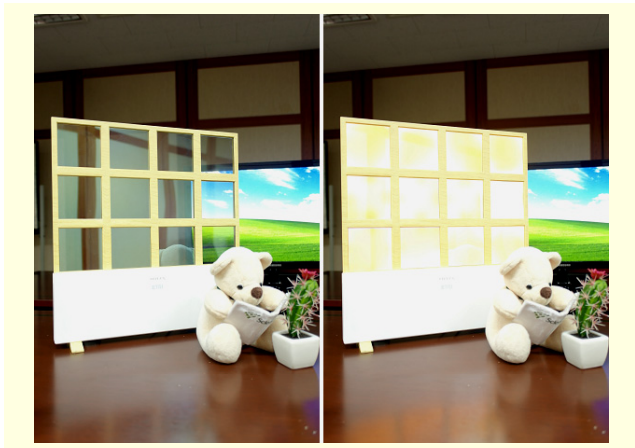
Fig. 8. Snapshot of transparent OLED lighting window.
